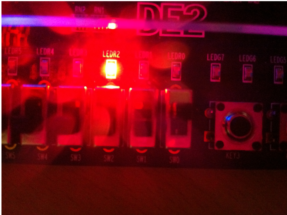
Figure 6: LED for the second state is turned ON after 1 second
