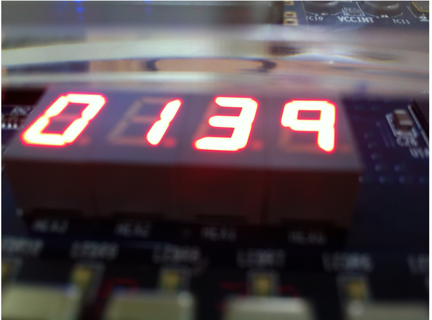
Figure 2: The left two seven segment displays are for seconds and the right ones are for the minutes
