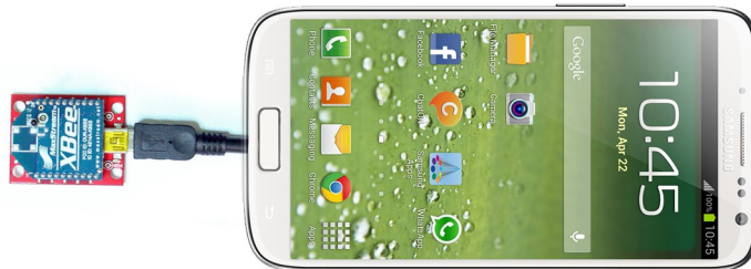
Figure 12: The figure shows one of the ways the smartphone can communicate with the AtMega328. The XBee module is attached using a USB cable to the smartphone and the XBee explorer which has FTDI chip on it, takes care of the conversion of data signals from USB to Serial.
