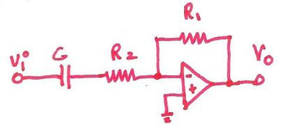
$$\omega_0 = \frac{1}{R_2 C} \quad H_0 = -\frac{R_1}{R_2} \quad |H_0| = \frac{R_1}{R_2}$$
