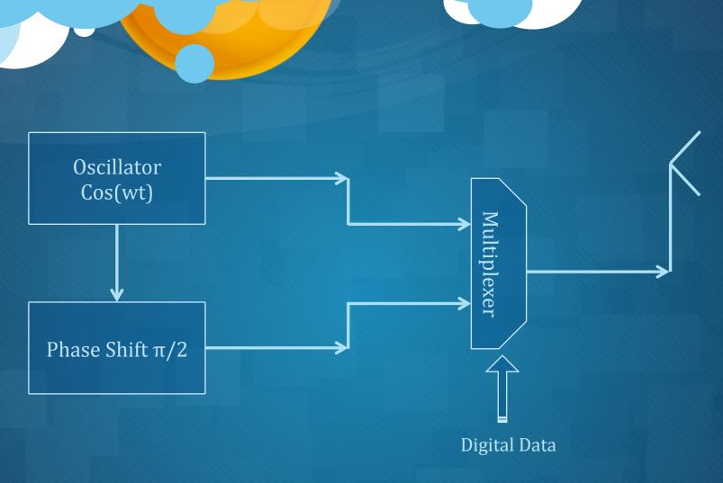
Multiplexer chooses the signal according to the digital data incoming and sends it to antenna.
