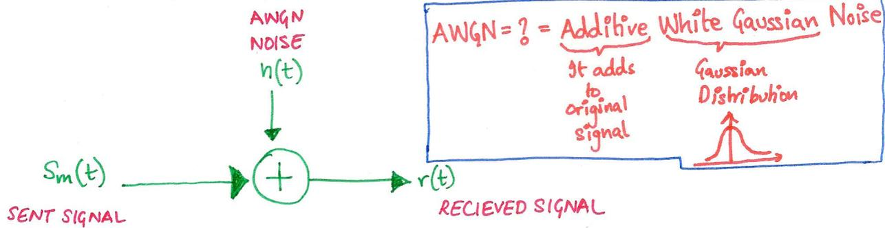
The AWGN,  $n(t)$  has power spectral density =  $\frac{N_0}{2}$  (Watts/Hz)
