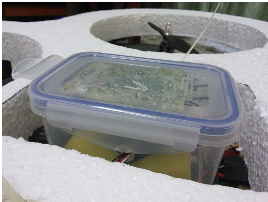
FIGURE 2.48: Protective Box Close Up
