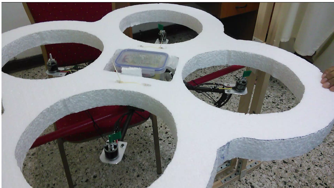
FIGURE 2.39: Prop-guard Built with Styrofoam
