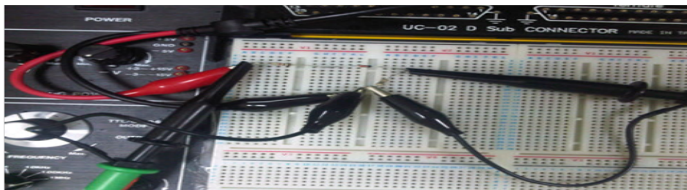
Figure 9: The connection for half wave rectifier
