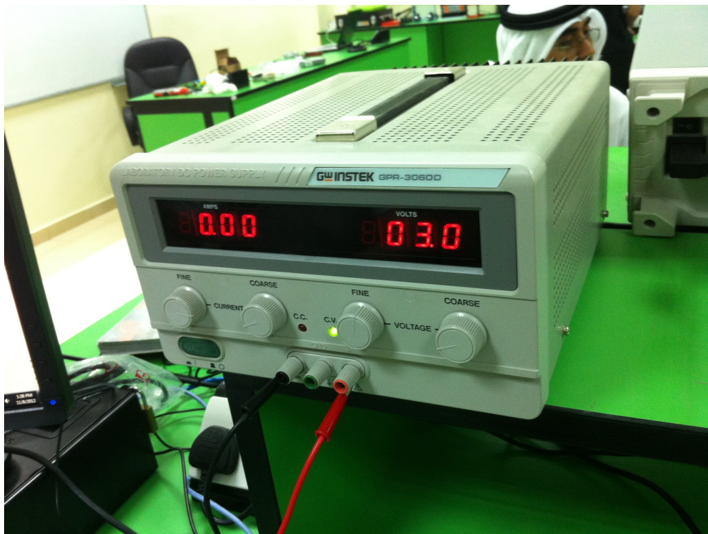
Figure 7: The DC power supply providing 3.0V constant
