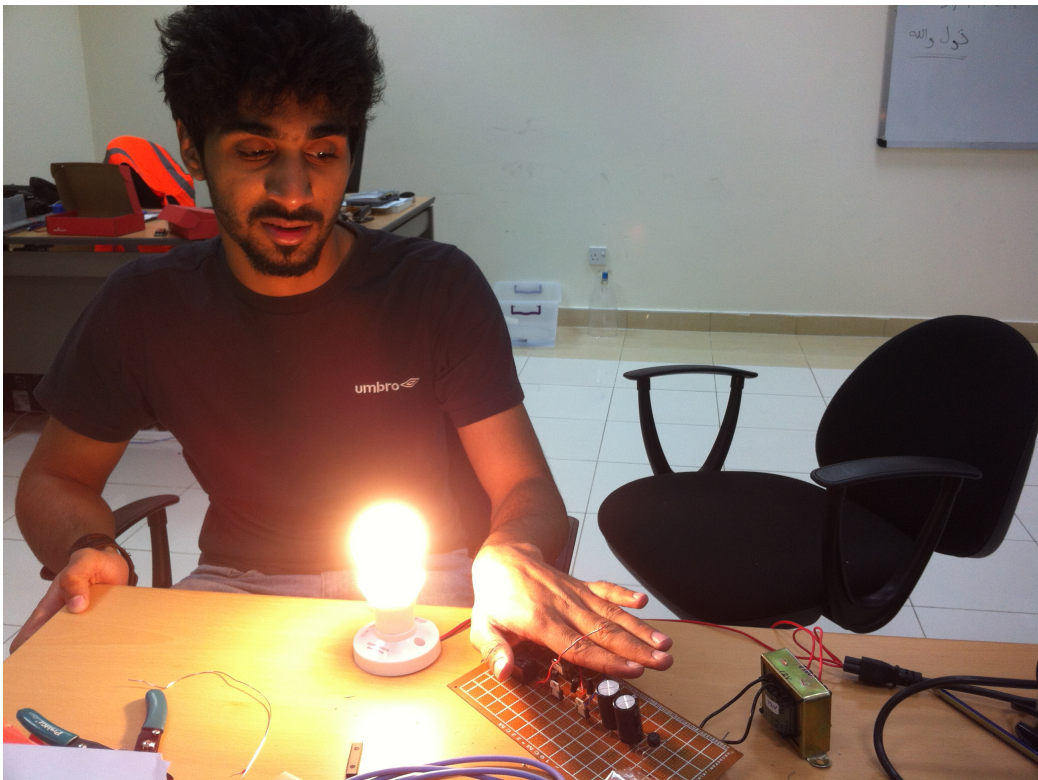
Figure 4: When LDR is not in light, the Bulb is ON
