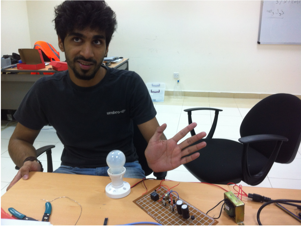
Figure 3: When LDR is in light, the Bulb is OFF
