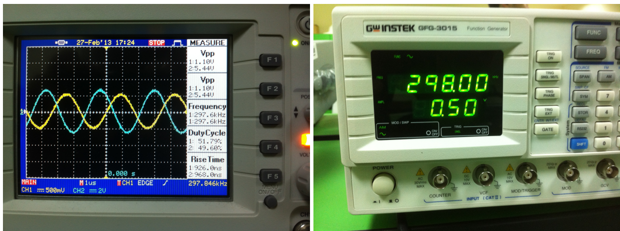
Figure 5: The Gain is there as the blue wave is higher in amplitude than the yellow (input) one Figure 6: Setting the frequency from the frequency generator as the input to the circuit
