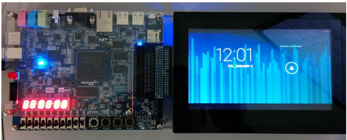
Figure 2: Android running on DE1 SoC Altera Cyclone V by University of Toronto.
