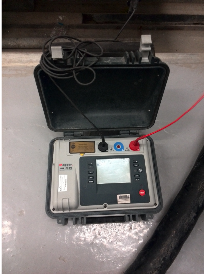
Figure 21: The figure shows the Megger 10kV insulation tester. This device is used to test the insulation of electrical component.
