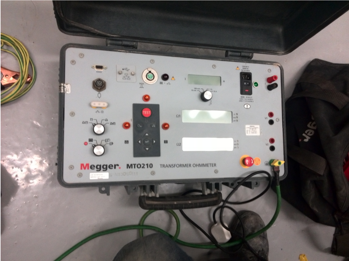
Figure 24: The figure the Megger Transformer Ohmmeter which is used to find out small resistances of transformers. The unit takes 240V AC supply and the test current can be selected through a knob from 10mA - 10 A. This test current is then passed through the winding and the resistance is calculated. The unit can also be connected through a USB cable to the computer for detailed analysis.
