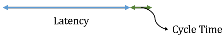
Figure 6: Data level parallelism. The time it takes for the first result to come out is called latency. But after that time the results are pushed out within one clock cycle.
